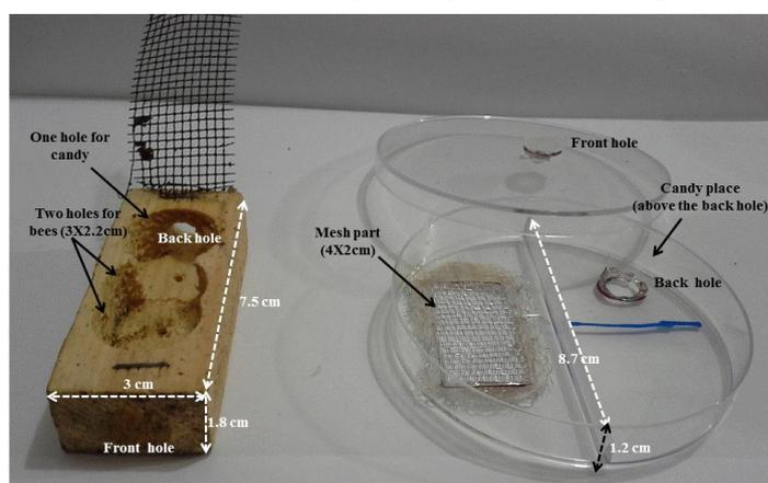
Fig. 1: Dimensions of traditional wooden cage and those cages made from modified plastic Petri dish.
